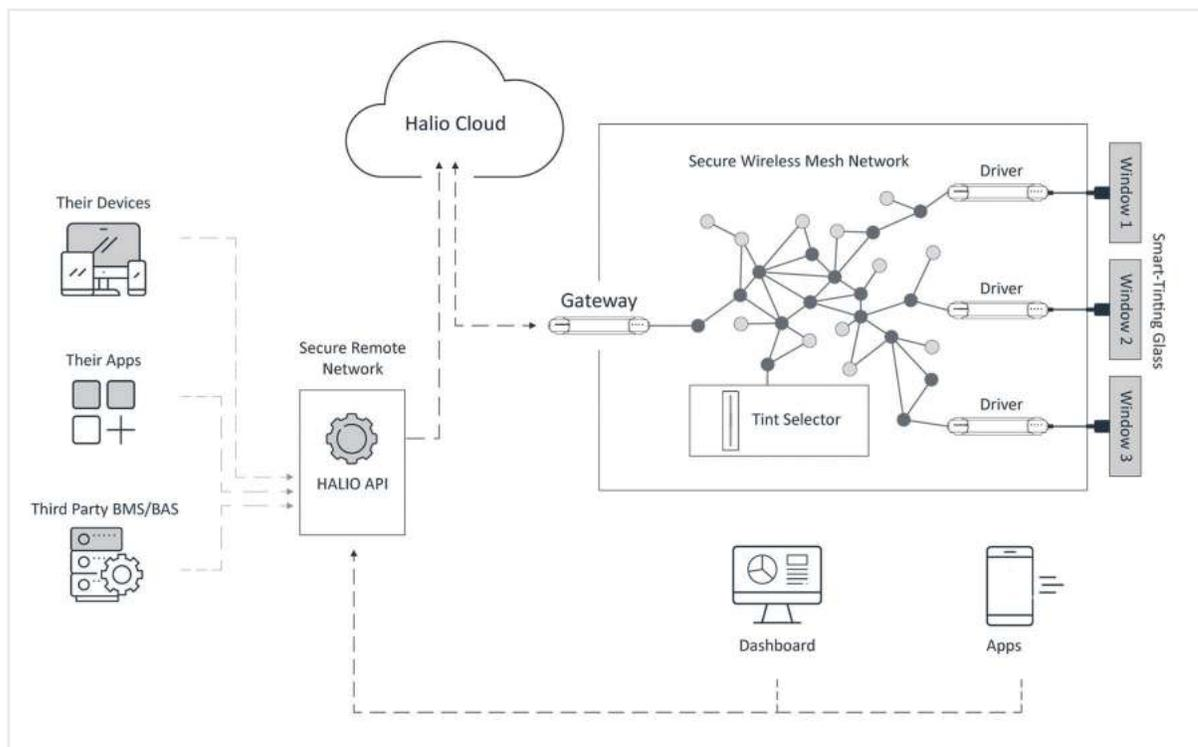
Figure 8: Example of a Halio network, including Halio Cloud, Halio Gateway, and the API
