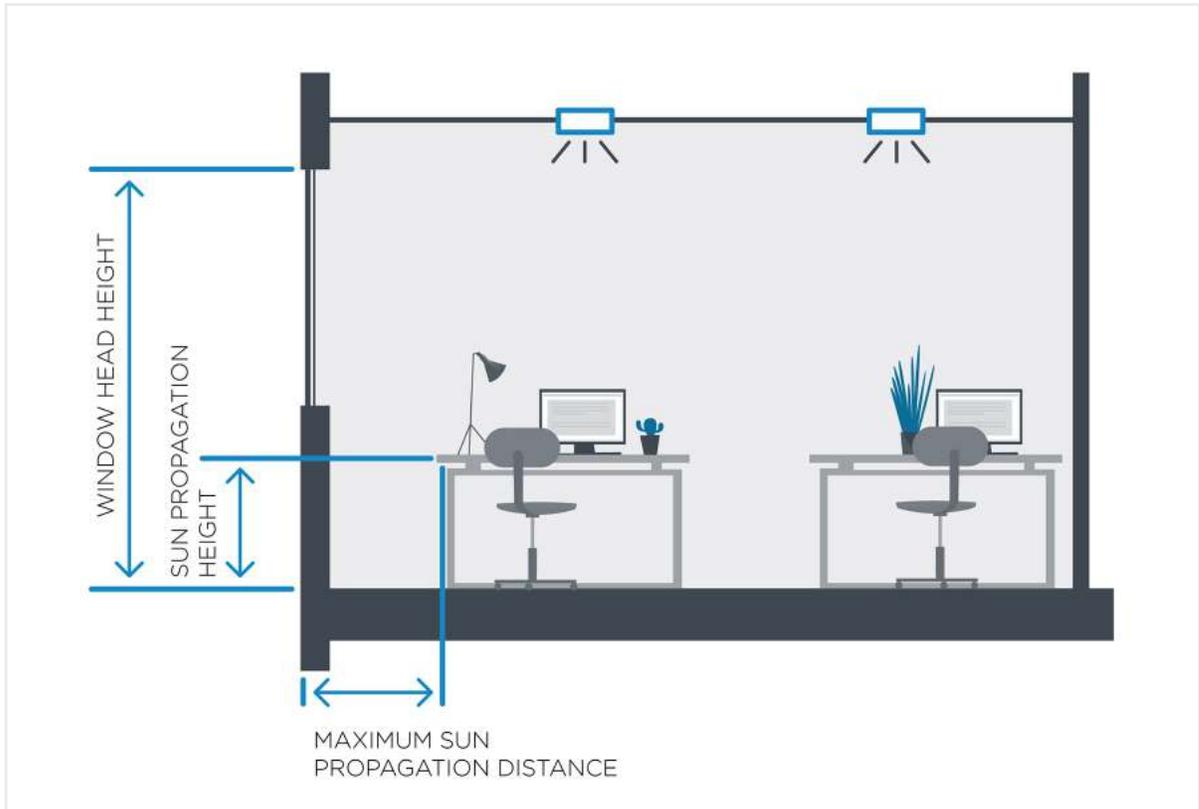
**Figure 7:** Determining maximum sun propagation distance
